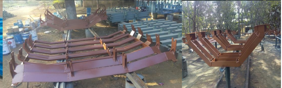
Standard idler base frames – Mass production on ROBOTIC Welding Machines
