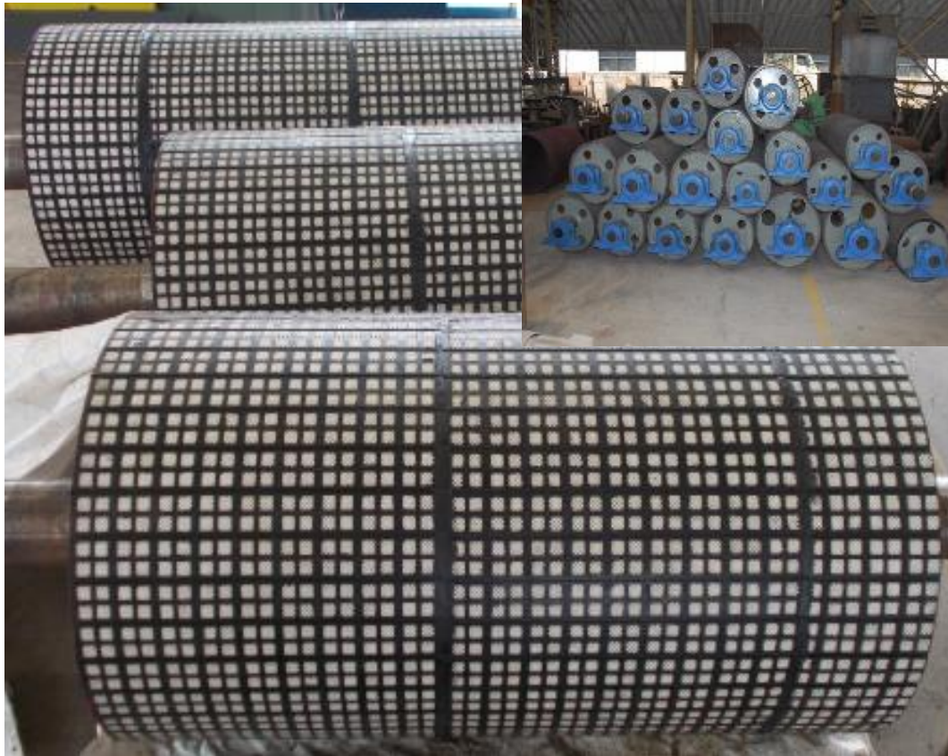
Pulley lagged with Ceramic Tiles
